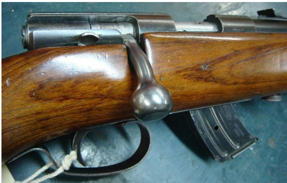
Figure 10. A SAF Slazenger Model 12 fitted with ten round magazine
