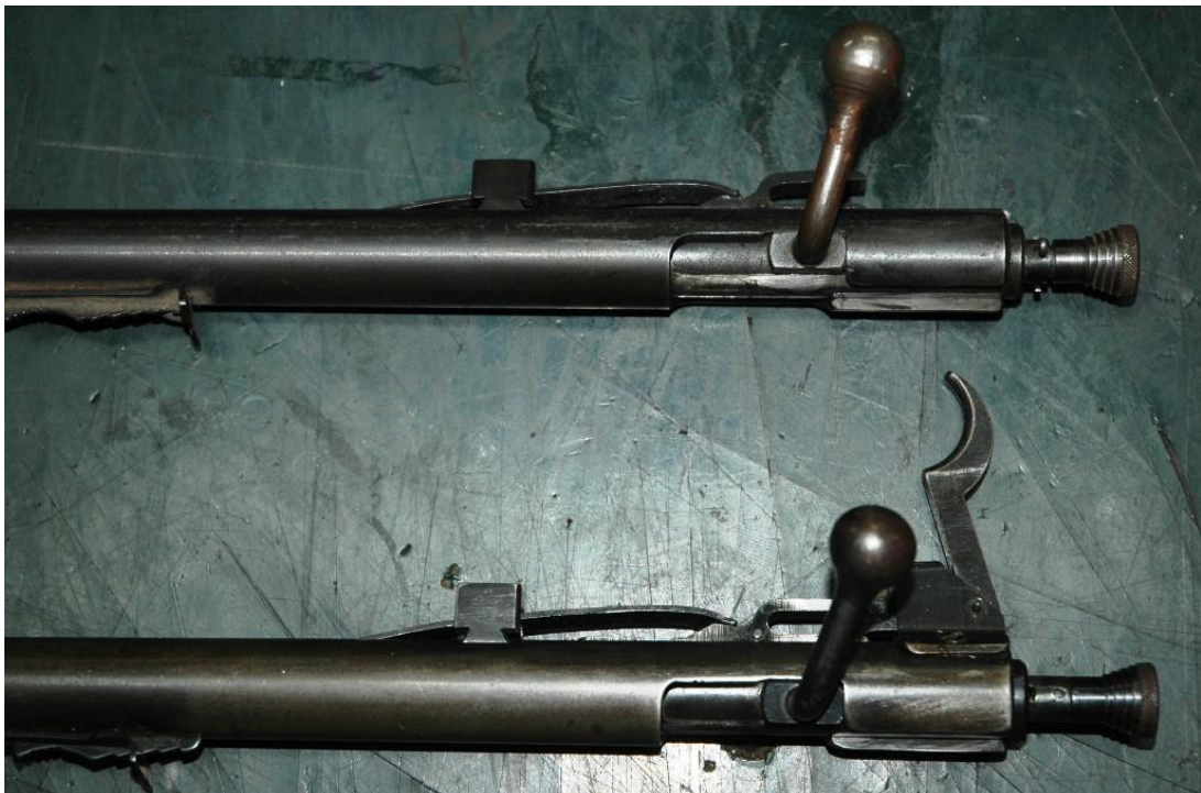
Figure 2. Lithgow SAF Model 1 (top) has the trigger attached to the stock whilst both the SAF Slazenger Model 1A and 1B (below) have the trigger assembly screwed
