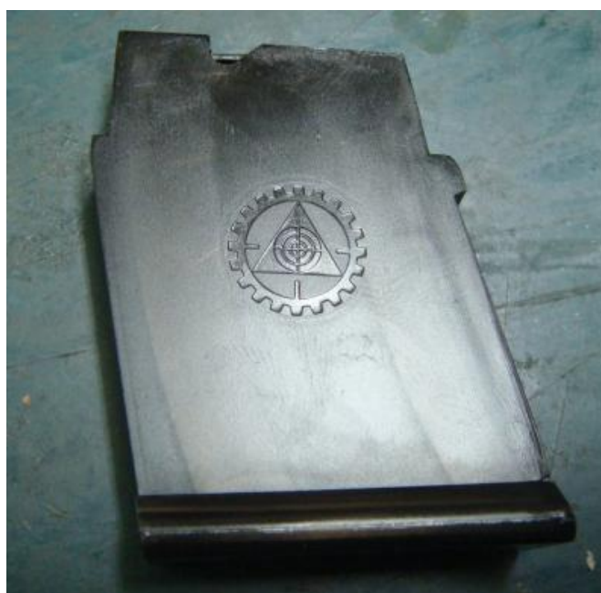
Figure 18. Lithgow Arms LA101 Crossover five round polymer magazine
