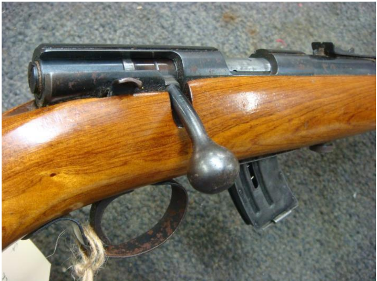
Figure 12. Lithgow SAF Slazenger Model rifle with ten round magazine
