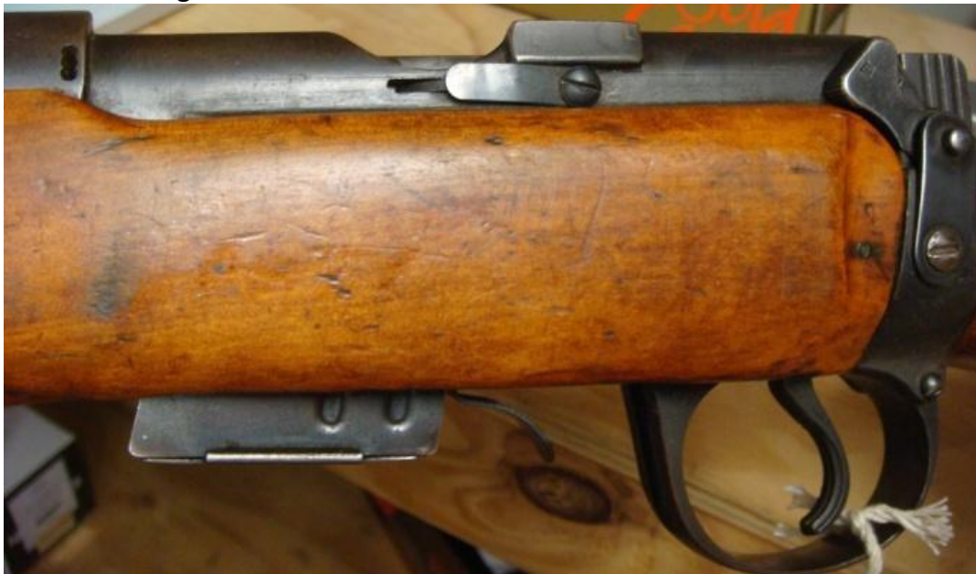
Figure 20. SAF Model 24 conversion to 22 Hornet calibre
