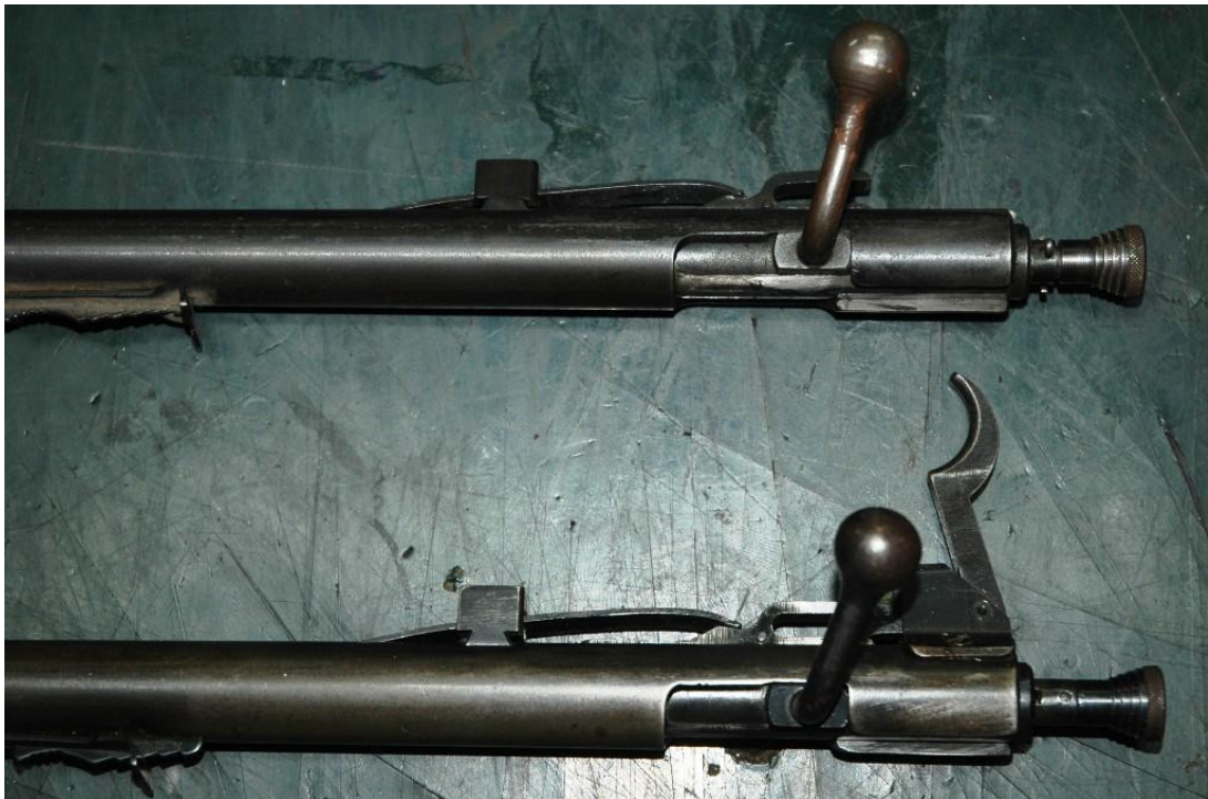
Figure 2. Lithgow SAF Model 1 (top) has the trigger attached to the stock whilst both the SAF Slazenger Model 1A and 1B (below) have the trigger assembly screwed to the barrel/receiver
