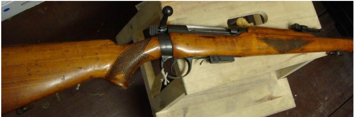
Figure 20. SAF Model 24 conversion to 22 Hornet calibre
